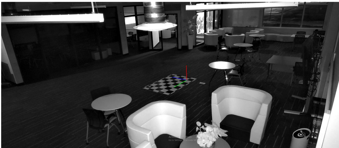
Figure 4: An example of the three axes being drawn at the origin of the calibration mat after pose estimation. The correct orientation and position of the three drawn axes ensure that there was a successful pose estimation. This also ensures that the position of the camera and rotation relative to the origin is accurate.
